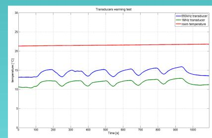
circulation system, sonication response stability and reproducibility up to 100% duty cycle, thus preventing gradients Warming test: 120 s, DC 100%, 5.5 W/cm<sup>2</sup>,  $\Delta T \sim 3$ °C.
