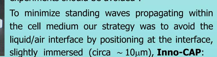
a cap of material which substantially matches the acoustic properties of the medium, and effectively allows US wave propagation to a phono-absorbant material.
