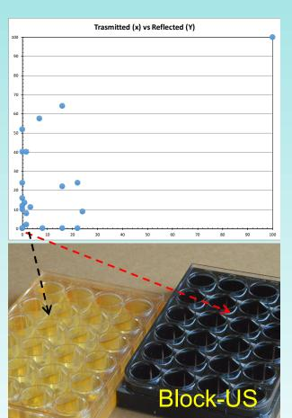
Measuring US transmission and reflection of a series (>50) of 1,00 MHz compositions, polymer composition named Block-US was identified. Measuring the sideleakage neighboring well acoustic using hydrophone @ 0°, 60°, 90° we estimated the amount of the attenuation of the wave mode conversions propagating in the sample.
