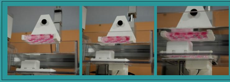
**Stable sample temperature:** ensured by a thermostated bath for cell culture, continuously degased to avoid both thermal and gas discontinuities
