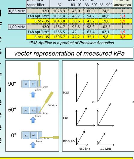
Block-US reduces 1.9 (0.65MHz) and 3.2-fold (1.0MHz) WMC propagation in side-wells
